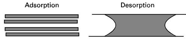
Figure 14 Schematic drawing of the adsorption layer in a cylindrical pore. (a) During adsorption from the laboratory air. (b) During drying of a previously water soaked sample.
